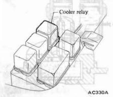
Fig. AC-34 Layout of Cooler Relay
