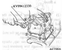
Fig. AC-76 Sequence of Removing Rear Cover Mounting Bolts
