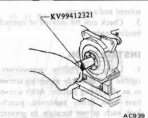
Fig. AC-68 Inserting Shaft Seal Remover and Installer
