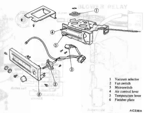
Fig. AC-43 Heater Control
