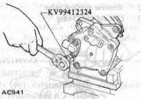
Fig. AC-74 Removing Discharge Value
