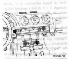
Fig. AC-41 Removing Heater Unit
