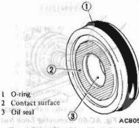
Fig. AC-71 Checking Shaft Seal Seat
