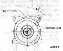
Fig. AC-88 Relative Position between Cylinder and Shell
