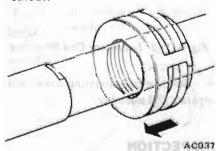
Fig. AC-72 Inserting Shaft Seal
