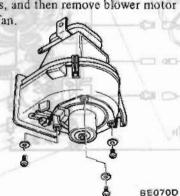
Assembly Fig. AC-51 Removing Blower Motor
