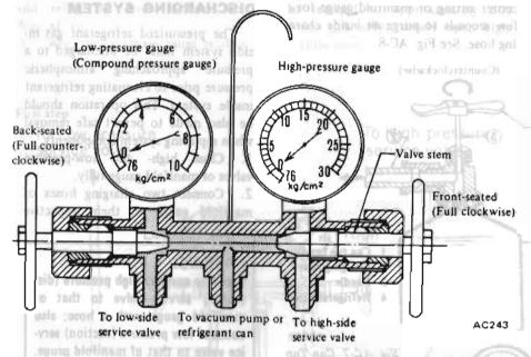
Fig. AC-5 Manifold Gauge
