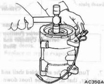
Fig. AC-83 Removing Front Cover
