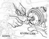
Fig. AC-58 Removing Clutch Hub
