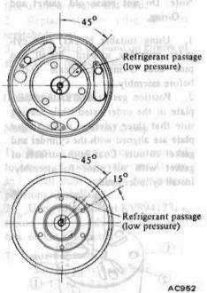
Fig. AC-86 Relative Position between Cylinder Head and Front Cover
