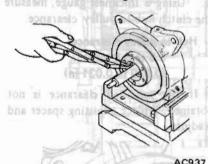
Fig. AC-66 Removing Retainer Ring
