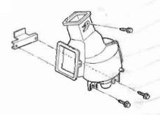
AC405A Fig. AC-50 Removing Blower
