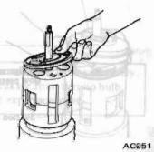
Fig. AC-85 Installing Cylinder Head
