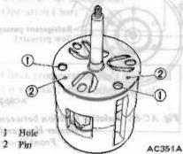
Fig. AC-84 Installing Suction Valve Plate
