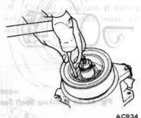
Fig. AC-63 Punch-Locking
