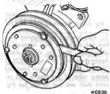
Fig. AC-64 Checking Clutch Hubto-Pulley Clearance
