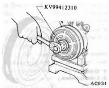
Fig. AC-60 Removing Lock Nut
