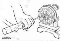
Fig. AC-59 Flattening Lock Washer Tab
