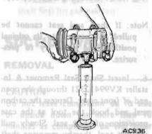
Fig. AC-65 Draining Compressor Oil
