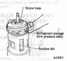
Fig. AC-87 Installing Front Cover
