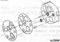
Fig. AC-79 Cutouts of Cylinder and Gasket
