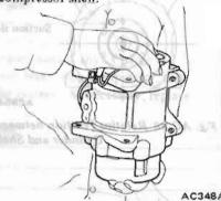
Fig. AC-81 Removing Cylinder
