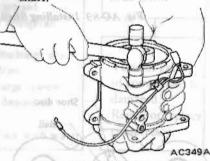
Fig. AC-82 Removing Cylinder Assembly
